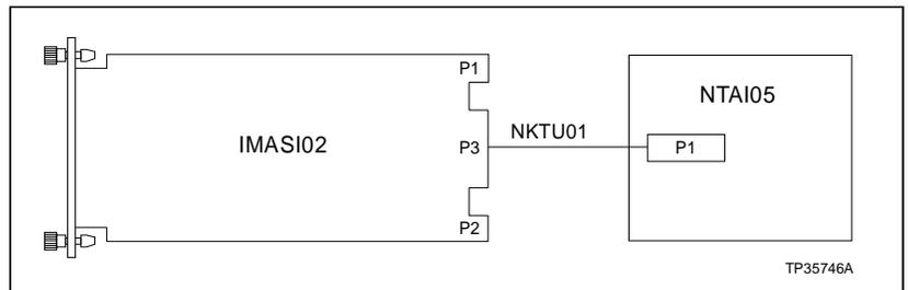
Figure A-4. Cable Connections for NTAI05
