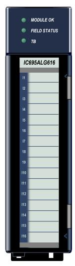
Non-Isolated Differential Analog Voltage/Current Input module IC695ALG608 provides 8 single-ended or 4 differential input channels. Non-Isolated Differential Analog Voltage/Current Input module IC695ALG616, shown at left, provides 16 single-ended or 8 differential input channels. Analog input channels can be configured for these ranges:
